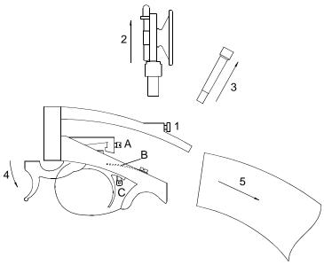
A = trigger adjustment screw
